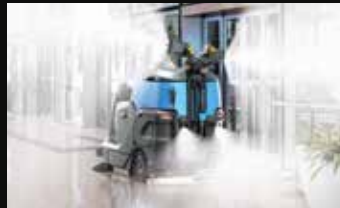
The Disinfector kit includes two groups of nozzles located above the tank for sanitizing vertical surfaces and a group at the base of the machine intended for the floor
